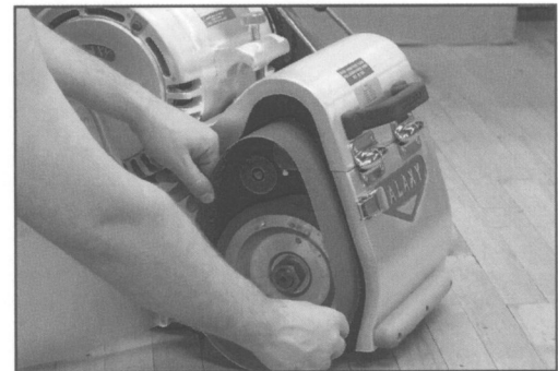
23. Slide belt into position.
