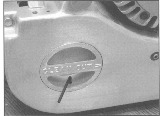
39. Use the key provided to remove dust cover.
